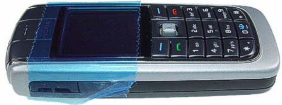
Protect the window with a plastic film.
