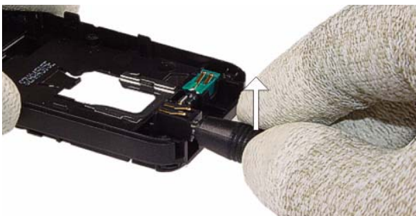
Remove the DC-jack with a DC-plug.
