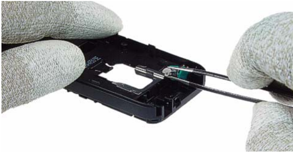
Lever out the vibra motor.
