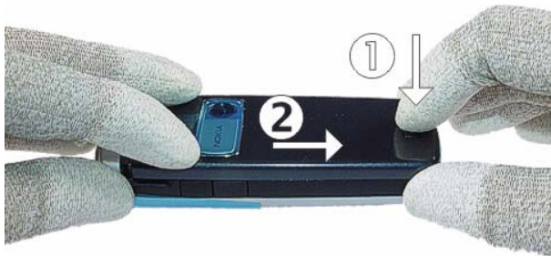
Remove the C-cover and protect the camera window.
