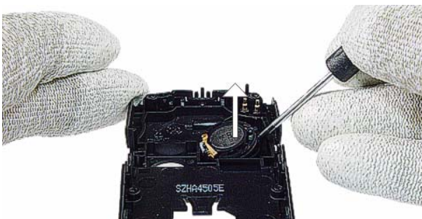
Release the IHF speaker carefully with a slot-headed screwdriver. Always use a new speaker adhesive when assembling.
