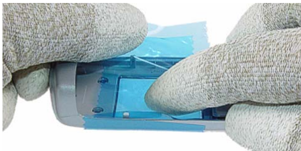
Also protect the inner side of the window with a protective film.
