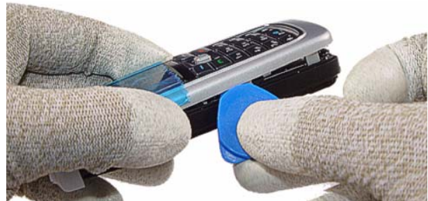
Unlock the side snaps with SRT-6 when opening the A-cover.
